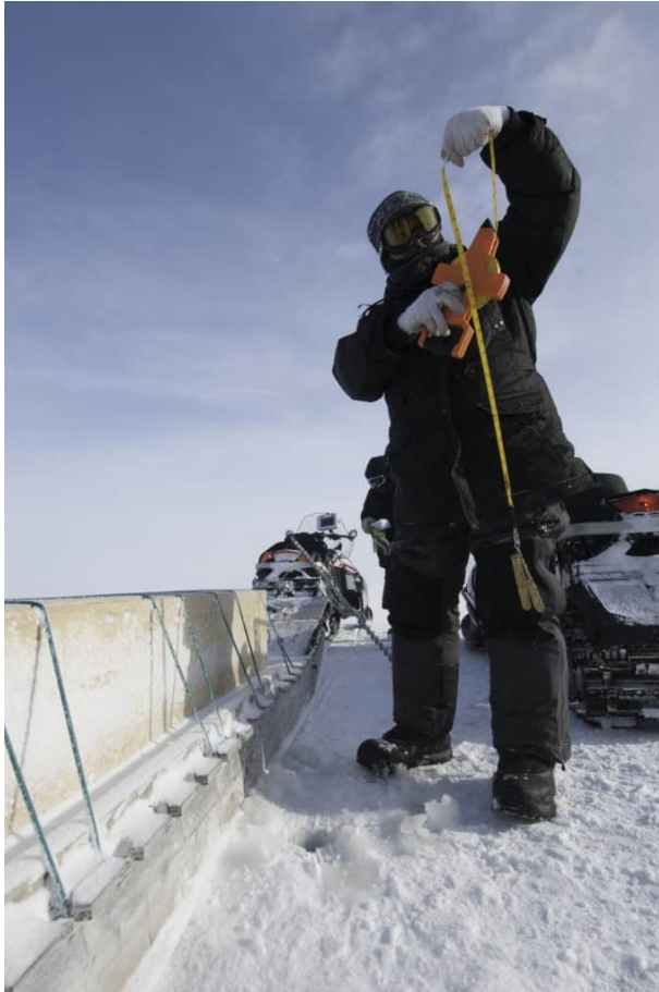
Figure 2 - Rex Holwell calibrates the SmartKamutik to ensure the radar reading and actual ice thickness are appropriate.
