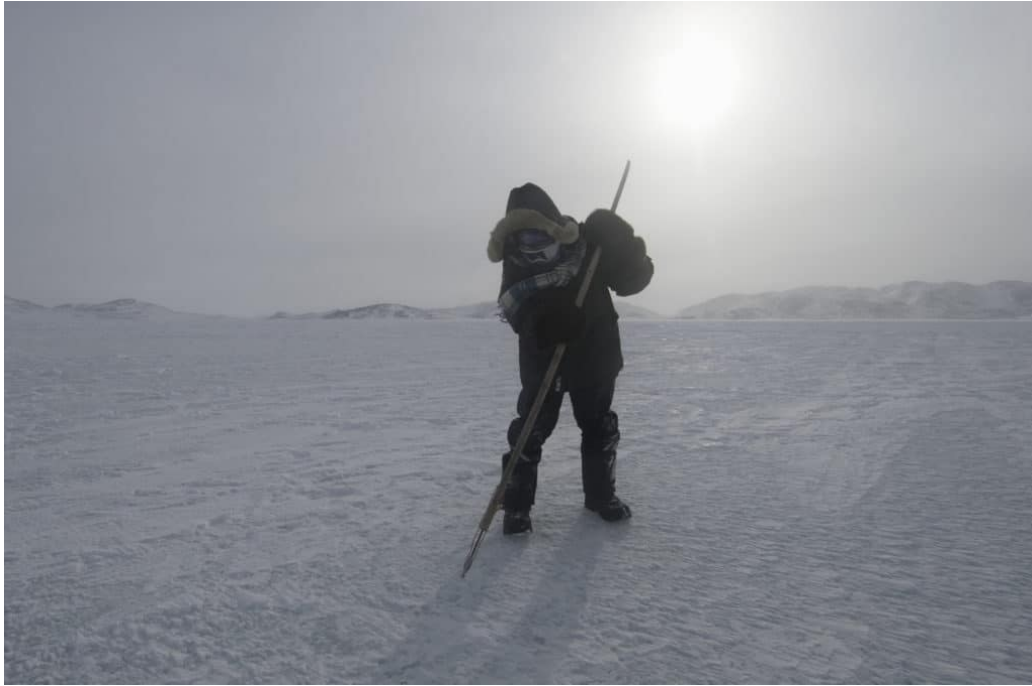
Figure 5 - Noah Noggasak demonstrates traditional use of a harpoon to gauge sea ice safety.
